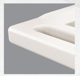
The attractive handrails integrated into the wash basin are hygienic because their rounded shapes are easy to clean. They are also safe for daily use as they have been tested with a constant load of 200 kg for one hour – far exceeding the market standard.
