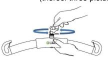
4. Does the sling bar attachment rotate with uneven or high resistance?
