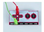
Finally, attach the other end of the alligator clip to the EARTH bar as shown.
