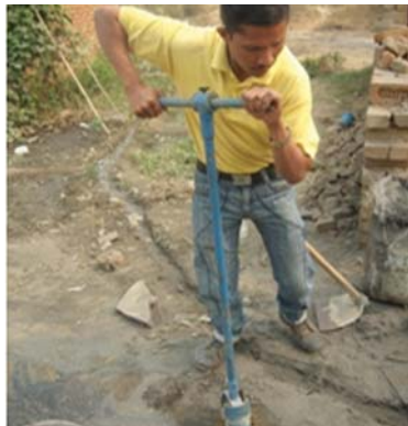
FIGURE 7 (Left) Soil sample collection in Loni area
