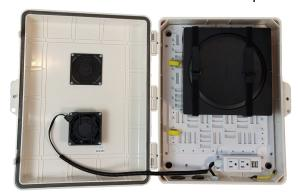
With this single-fan (active intake) configuration example shown below, we have a Sonos Amp secured with enough room for wire management, we even have enough space for another small device, such as a streaming media player, network switch, etc.
