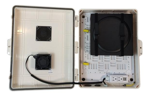
There is no wrong way to secure your equipment; you just must ensure the device and straps do not interfere with the full closure of the Shell, operation of the fan, or that it inhibits the airflow.
