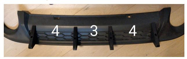
2. Place the first fin (outer) as shown in the picture below. Ensure that the step on the fin is pressed against the lower edge of the honeycomb grill edge.
