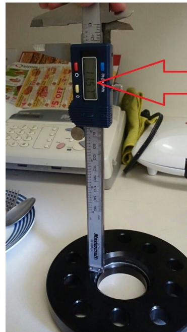
SPACER HUB CLEARANCE IS DEPENDENT ON THE SPACER THICKNESS AND HUB SIZE
