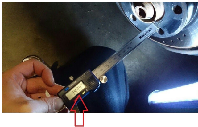
MEASURE HOW FAR THE HUB LIP STICKS OUT, SPACER SHOULD HAVE THE SAME OR MORE CLEARANCE BEHIND THE SPACER HUB
