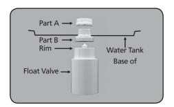
Part A and B must be tighten tightly together.
