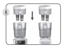
Place the inner container back into the outer container. Fill in water and flush out the first one or two rounds of filtered water.
