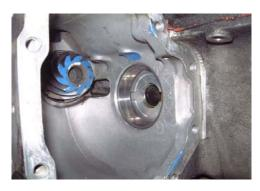
3. As shown in the image on the above, shave a little of the blue parts before placing the differential in the case, and shave more if the differential hits. Depending on the differential case, areas other than the blue parts shown may hit so be aware of this. Once this process is done, make sure the shavings are cleaned out properly.
