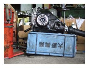
You need to change the oil after 3000km of OS Super Lock LSD installation. After that, please change the oil every 20000km. (This information is based on conventional street drive. If you drive in severe condition such as race condition, you may need to change the oil per race.)
