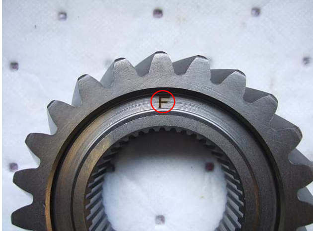
Pic 1. 4th Main Gear installation
