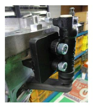
Step 11: Please connect the newly purchased OEM clutch line (**30855-CD00A**) and reinstall the transmission. Please bleed the hydraulic system as needed and confirm working operation.
