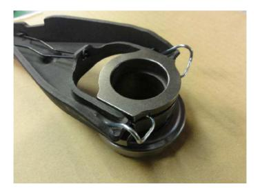
Step 9: Please install the newly assembled fork assembly into the transmission bell housing.
