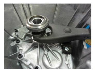
Step 10: Please mate the slave cylinder to the clutch fork. Adjust if necessary.
