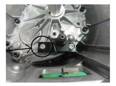
WARNING: Please notice the bolt circled. To prevent transmission fluid leaks from this bolt location, please be sure to apply silicone liquid gasket to the bolt threads to properly seal this location.
