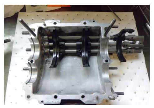
Caution: Desirable bolt tightening torque is 2.0kg
