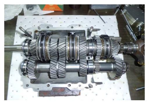
**Caution:** Once the installation is complete, please rotate the gear kit by hand to make sure it rotates smoothly without any interference.
