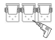
Note: Leave at least 2 inches higher than the ground for easier filter replacement.
