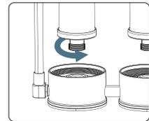
Step 3: Install back the filter housing.
