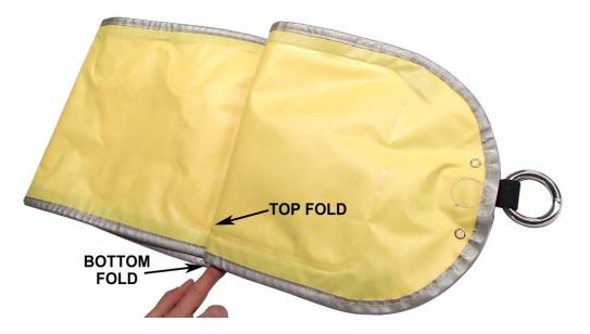
9. Fold the device over at this point. The inflator and cylinder should now be on top. If not, flip the device over.
