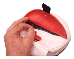
CAUTION: Do not remove the items inside until the inflation cylinder has been removed. Failure to remove the cylinder may cause an inadvertent inflation.
