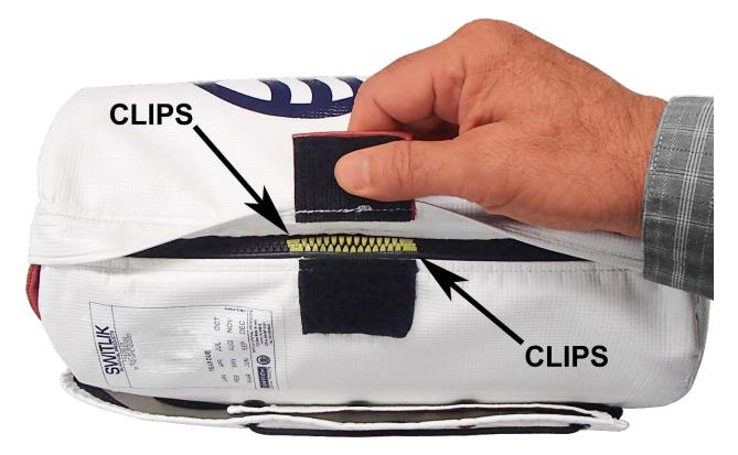
13. If the zipper has separated, pull the zipper slider back down past the Quick-Burst section, then pull it all the way back up. This will join the Quick-Burst clips back together. Close the cover over the Quick-Burst section and snap the top cover flap closed.
