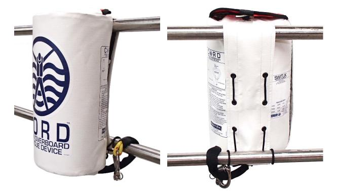
To secure the **CORD** to the rails, fully unlace the lacing flap. Place the flap over the top rail (or lifeline) and lace the flap back up. Note the lacing pattern below.
