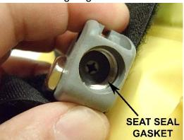
lower gaskets must always be replaced if the hex cap nut is loosened. These gaskets are included in the **CORD** rearm kit.
