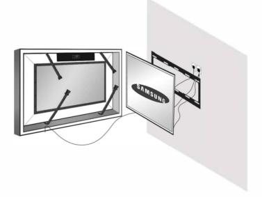
Rest the top side of the frame on the top edge of the TV and adjust to the left or right until the frame opening is centered with the screen.
