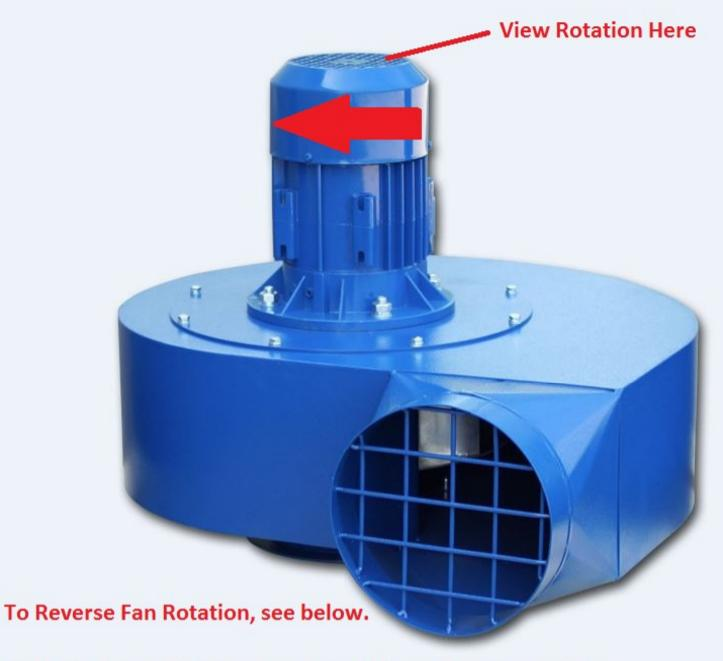
3 Phase Electrical - Interchange Any 2 Incoming Power Wires (e.g. - interchange Line1 & Line2)
