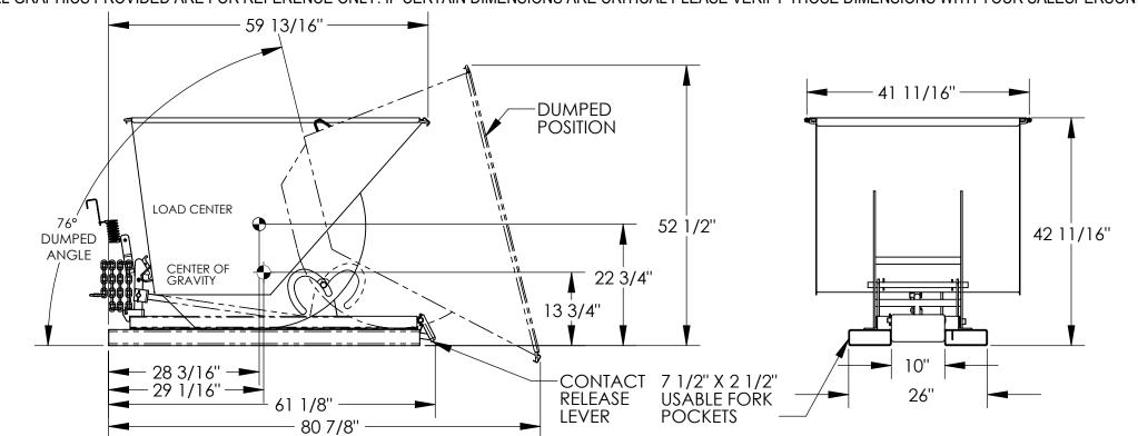
MODEL NUMBER: D-100-LD VOLUME: 1 CU. YDS. CAPACITY: 2,000 LBS. OVERALL WIDTH: 41 11/16"
