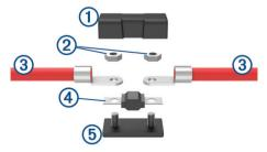
2 Using an 8 mm (<sup>5</sup>/<sub>16</sub> in.) wrench, remove the two nuts ② that secure the two parts of the power cable ③ to the in-line fuse assembly.
