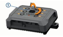
2 Pull the front cover off of the device.
