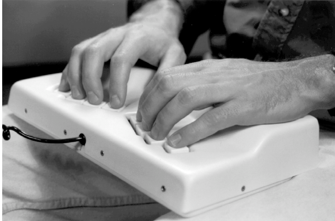
Figure 9. The Accukey a.k.a. Ternary Chord Keyboard (TCK) (used with permission, AccuCorp, Inc.).
