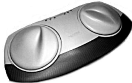
Figure 1: The AID-CTS keyboard for use by individuals with upper extremity disability.
