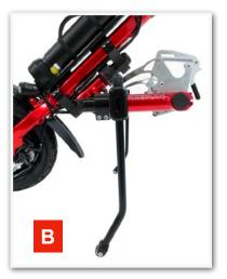
Push the kickstand clamp up against the coupler clamp "C". Tighten the screws loosely at first using your 4mm hex wrench. Fully tighten down the screws in a diagonal configuration. If the clamp pulls too close on one side, back off that screw and cinch down the remaining screws with more tension.
