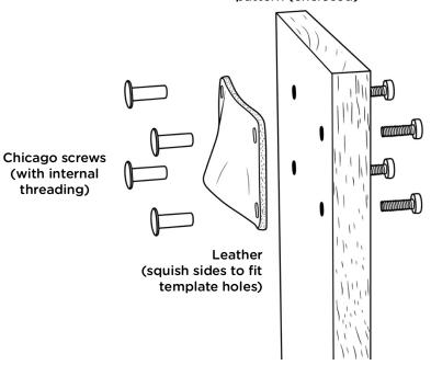
Back screws (different lengths for different cabinet widths)
