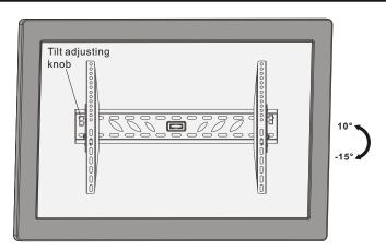
Loosen the adjusting knobs to tilt the TV to obtain desired angle then tighten them.
