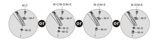
Note: Choose the appropriate screws, washers and spacers (if necessary) according to the type of screen.
