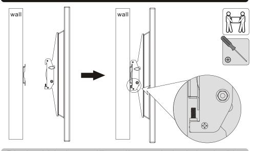
Tighten the two bolts by using a proper phillips screwdriver to secure the adapter brackets to the wall plate.
