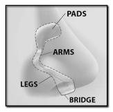
OUTWARD PRESSURE OF PADS INSIDE NOSE OPENS AIRWAYS
