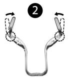
Bend top of PADS inwardly bending at pivot joint of ARM & PAD (at circle)
