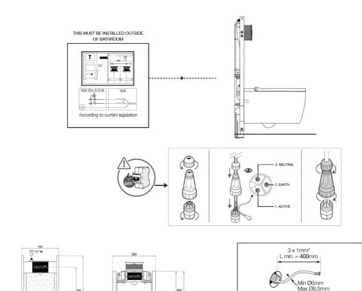
IPx4 400 mm (L) Power Supply must be firmly grounded.
