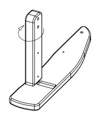
**6.** Rotate Part E clockwise until tight in the orientation shown
