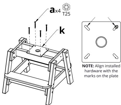
**4.** Attach Hardware k to the previous assembly using Hardware a
