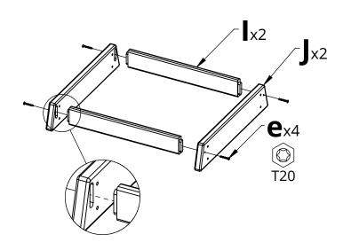
**1.** Connect Parts I & J together using Hardware e
