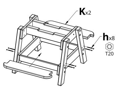
**3.** Attach Part K to the previous assembly using Hardware h
