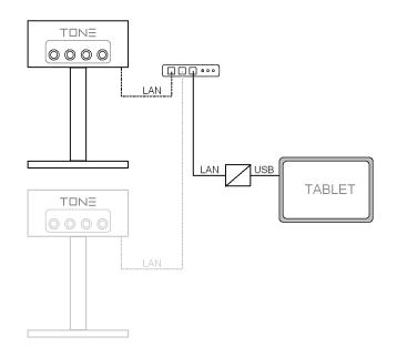
You need a LAN switch or router (#650310) and a LAN-2-USB converter (#650309) (router pre-configured by TONE) and a TABLET computer (#650308)
