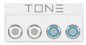
Buttons 3 & 4 light up blue -> No flow / water supply interrupted (Heating element can overheat) Flow meter defective
