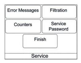
Press "Error Messages" to display a historical list of error messages. Some errors may be intermittent due to various conditions and do not necessarily cause the brewer to shut down. Press "Reset Errors" to reset the error count to zero. Press finish to return to the service screen.
