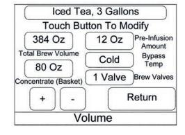
To modify the numeric values shown, first select an item and then use the + and – keys/buttons to change the value. Tap the non- numeric items to toggle through the available choices. When the preferred option is displayed, it is set. Brewers may not have componentry installed for all options. Items will be greyed out if unavailable due to other selections or values. Press return to return to the 'recipe settings' screen.
