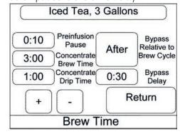
bypass water will be delivered during any concentrate off time available during the concentrate delivery. Note: A recipe made up of entirely cold water dilution (such as for making lemonade from concentrate) would cause all values on this screen to be greyed out as none of the items would be applicable. Press return to return to the 'recipe settings' screen.
