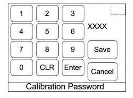
The calibrate screen will display. Items that are not installed or that have been disabled in the parameters section will be greyed out. Other items may be calibrated to ensure brewing accuracy. Only the items for which calibration is desired need be addressed.
