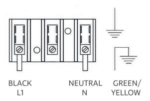
**NOTE:** This electrical service consist of 2 current carrying conductors (L1 and Neutral) and a separate conductor for earth ground.
