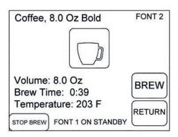
The screen at right shows a brew in process on Font 2 while Font 1 is idle. The "Stop Brew" key may be used to cancel the brew on Font 2. A brew process could be started on Font 1 without disrupting the brew on Font 2 if desired.
