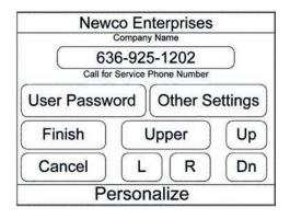
A 'service telephone number' screen with keypad will be displayed. Key in the service area code and phone number. Press Save to store the service telephone number. CLR will clear entry without exiting the screen. Cancel will exit the screen without saving changes and return you to the 'personalize' screen shown above.
