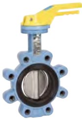
1181 - Disc CF8M up to DN100, Disc GGG50 epoxy coated above / Seat NBR For gas - PS: 5 bar (class MOP5) - TS: -20°C/+60°C.
