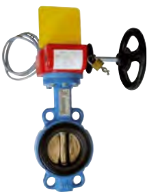
1142/1148 - Disc CF8M up to DN100, Disc GGG50 epoxy coated above / Seat EPDM For fire network - Acc. to APSAD R1 - With gearbox (& limit switches for 1142) - TS: -10°C/+110°C.
