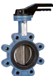
1163 - Disc CF8M / Seat EPDM TS: -10°C/+110°C.
