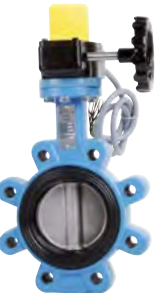
1182 - Disc CF8M up to DN100, Disc GGG50 epoxy coated above / Seat EPDM For fire network - FM approved - With gearbox & limit switches - TS: -10°C/+110°C.
