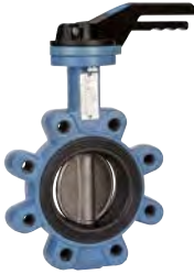
1162 - Disc CF8M up to DN100, Disc GGG50 epoxy coated above / Seat NBR TS: -10°C/+90°C.
