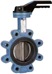
1164 - Disc CF8M / Seat FKM TS: -5°C/+180°C.
