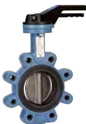
1160 - Disc CF8M up to DN100, Disc GGG50 epoxy coated from DN125 to DN300, Disc GGG50 rilsan coated above / Seat EPDM TS: -10°C/+110°C.
