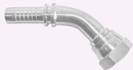
45° SWEPT SWIVEL ELBOW 60° CONE BSPP FEMALE
