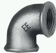
90° REDUCING ELBOW BSPP FEMALE
