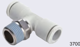
MPT BSPP SWIVEL BRANCH TEE WITH O-RING
