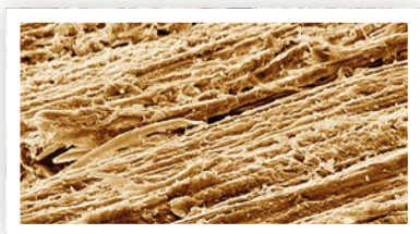
» Wooden surface after sanding with aluminium oxide.
