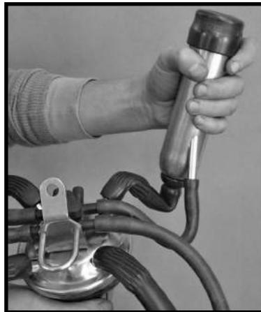
Left: When Shut-Off Button is pushed UP the claw is open, and vacuum is allowed through the claw and inflations.
