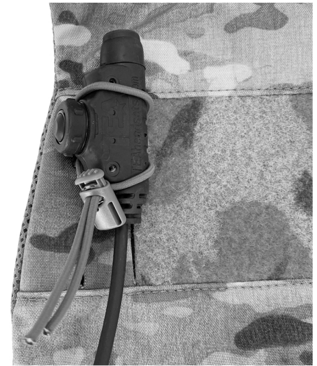
VERTICAL MOUNTING IN VERTICAL SLOTS/ MOLLE WITH A PTT SHOWN AS AN EXAMPLE. CORD LOCKS OR KNOTS CAN BE USED FOR ADJUSTMENT OR SECURING.
