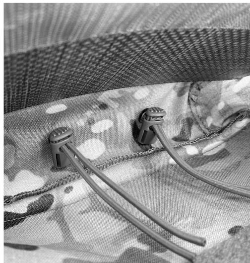
MOUNTING THROUGH GROMMETS/ EYELETS ON POUCHES. INSIDE OF A POUCH SHOWN. CORD LOCKS OR KNOTS CAN BE USED FOR ADJUSTMENT OR SECURING.
