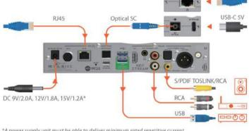
\*A power supply unit must be able to deliver minimum rated repetitive current.
