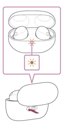
3 Release your finger within 5 seconds after the indicator (orange) on the charging case starts flashing.
