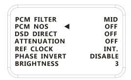
Default is OFF. Turn on to bypassing the internal interpolating FIR filter. The raw PCM stream is sent into the R-2R ladder directly.
