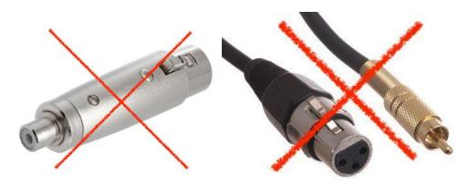
Therefore, please only use the custom-made, Burson-marked XLR-RCA adapter we have provided in our accessories box to connect the XLR outputs of our products to any downstream amplifiers with RCA inputs.
