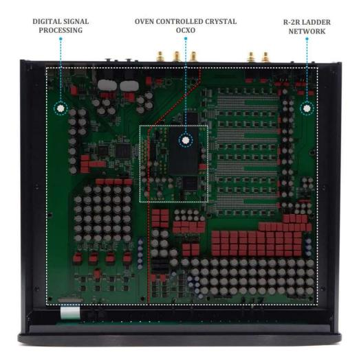
**DIGITAL SIGNAL PROCESSING** – All digital input data are stored in the on-board FPGA high-speed RAM.
