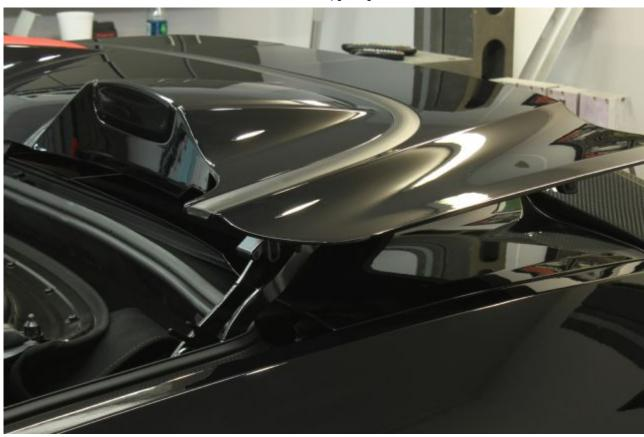
**03.** The first step in the project simply involves pushing a button. With the top lowered, push and hold the top's power button until the tonneau cover extends to approximately the position shown here. Releasing the button holds the top in place.
