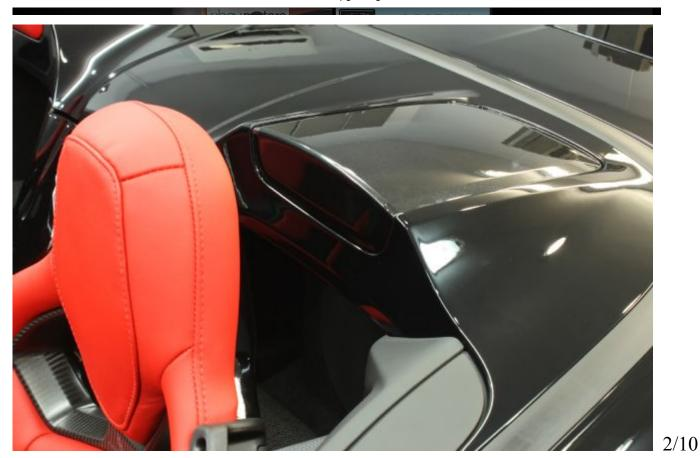
**01**. Chevrolet could have molded the C7 convertible's tonneau cover as a single piece, but thoughtfully added the body-color, composite inserts behind the headrests as a nod to the personalization they knew owners would appreciate.
