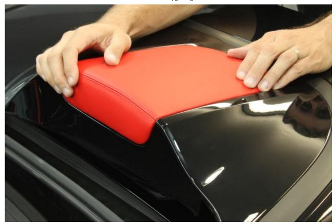
**06.** Now, it's simply a matter of dropping on the new inserts and reusing the nuts to tighten them onto the tonneau cover. A light application of muffler oil can be used to lubricate the studs, if necessary. Job done.
