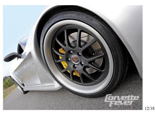
Form Follows Function, While Filling the Fenderwells::: As with the rest of the car, if stock C6 components are good, the C6 GTR upgrades are even better. Michelin Pilot Sport ZP rubber graces either HRE or Forgeline (seen here) alloy wheels, which bolt onto massive Stop Tech discs.
