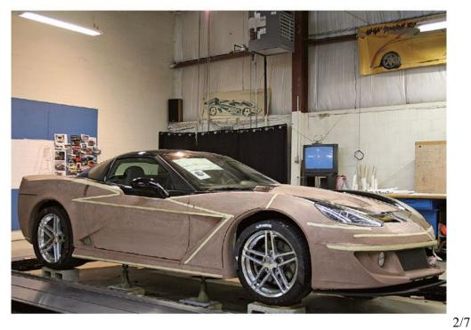
At Specter Werkes/Sports' Troy, Michigan, studio, the GTR's bodywork is shaped in clay. When finalized, the clay form will serve as the model for new fiberglass panels. Almost every body panel on the car will be replaced.
