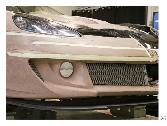
One of the most distinctive styling elements of the new GTR is a more pronounced lower front fascia with fog lamps, a larger grille opening, and brake-cooling ducts.
