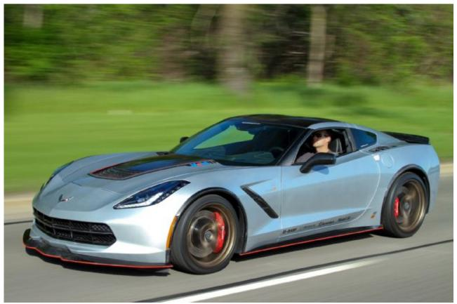
The wicker on the rear spoiler, for example, offers 25 mm of vertical adjustment, enabling fine-tuning for the requirements of different tracks, while the wheelhouse extensions provide the necessary coverage for wider wheels and tires. The Concept7 cars Nowicki has built to date have worn 275/30ZR19 front and 305/30ZR20 rear Michelin Pilot Super Sport tires, all riding on custom HRE P101 19x9.5 front and 20x11 rear wheels.
