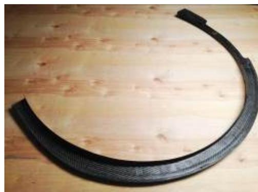
away from the edges of the part. That will help prevent it from squeezing out onto the body when it is installed.
