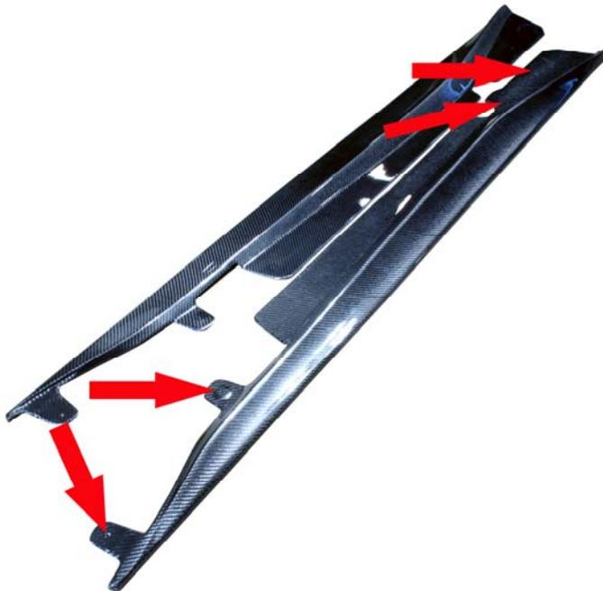
3. Re-install the previously removed 7mm screws and tighten them.
