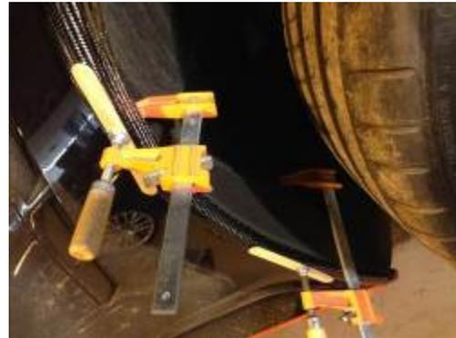
2. When the flare's installation position is determined, scuff the portion of the fender under the flare with a 3M Red pad to ensure proper bonding with the adhesive.
